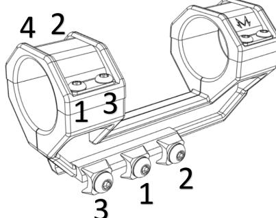
Make sure lugs are engaged to rail & washers are in place and torque to 25 in-lbs dry. ¼ turn at a time in sequence shown above.
